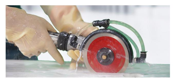
The finished product is an inert, stable product that does not release hazardous materials in its fully intact form. Therefore, it is advisable to carry out all processing and fabrication tasks in the factory to avoid generating silica dust at the installation site.
